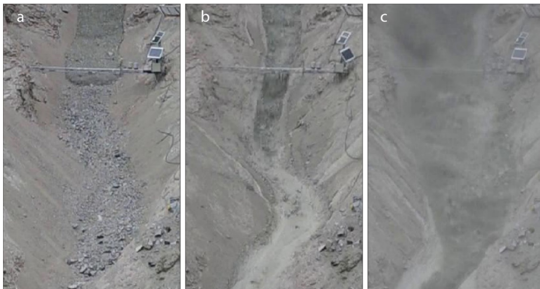
Fig. 2. Representative examples of debris-flow surges with different sediment concentrations estimated qualitatively from video. (a) High-sediment (Low-water) concentration; (b) Intermediate-sediment concentration; and (c) Low-sediment (high-water) concentration. In general, sediment concentrations decrease with increasing rainfall intensity.
