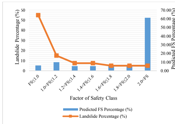
Fig. 6 Results obtained by TRIGRS in each class; the graph of the Landslide percentage and the predicted FS percentage vs. factor of safety class.
