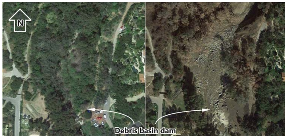
Fig. 2. Google Earth images of the San Ysidro debris-catch basin at the mouth of the range front approximately 360 meters upstream of East Mountain Drive. Image date April 14, 2017 (left); January 12, 2018 (right). © Google Earth (both images).
