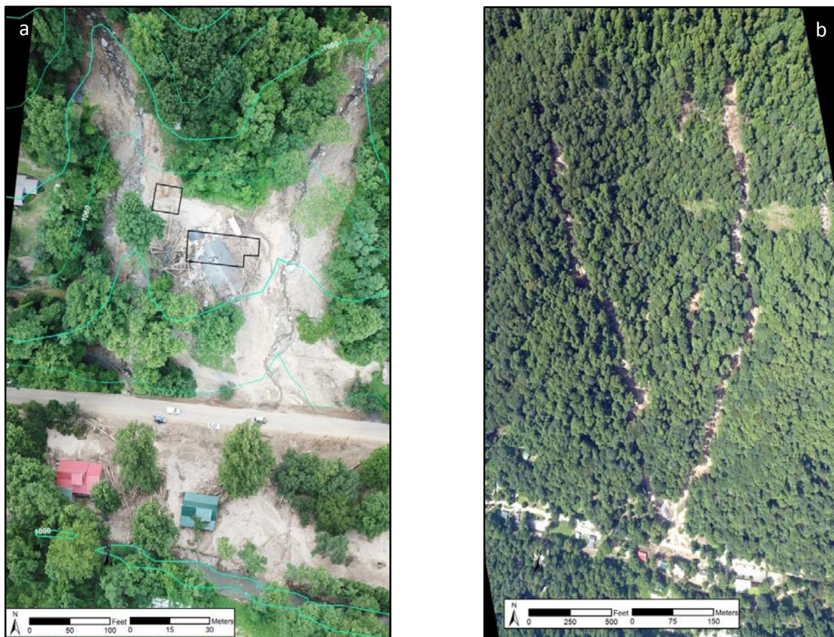
Fig. 3. (a) Georegistered 2018 UAV Image from the NC Geodetic Survey. Original location of Case home and detached garage outlined in black. (b) Georegistered 2018 Aerial Image from the NC Forest Service. Two debris flows that merged at the base of Little Warrior Mountain at the Case home location along Highway 176.
