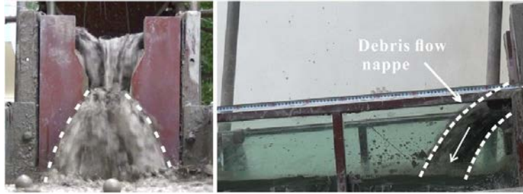
(b) Debris flows passing through spillway with "Y-type" cross-section
