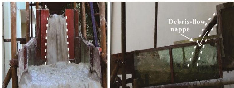
(a) Debris flows passing through spillway with rectangular cross-section
